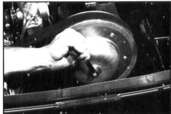
5. Remove three mounting bolts (A, B, C) securing chaincase to chassis. Carefully tip machine on its left side onto a mat. Lift chaincase up until drive shaft is out of lower chaincase bearing. Lift drive shaft up until it clears tunnel on LH side (bottom) and can be pulled out of tunnel. Remove drive shaft and track.
